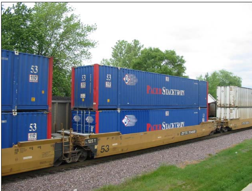
Figure 4: A Double-Stack Car owned by the TTX Company
