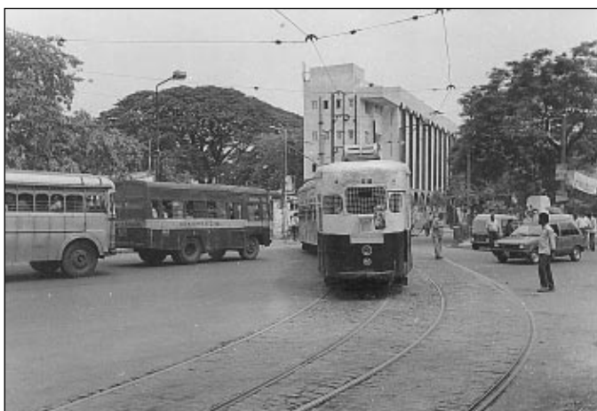
Car no. 347 (English Electric, 1931) negotiating a curve. Pre-war trams still provide the backbone of the system
